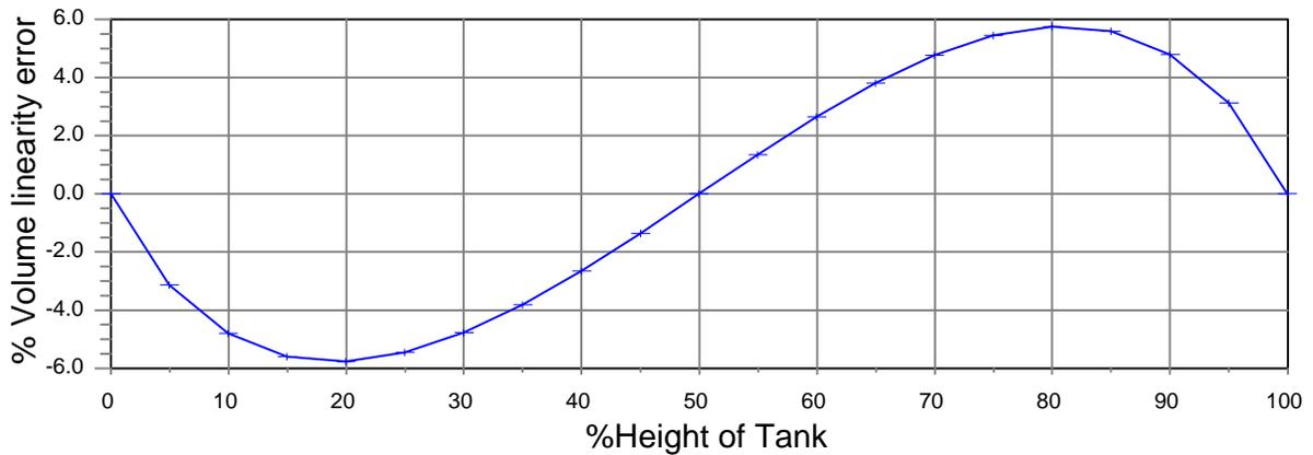
Graph 2b: linearity error of a horizontal tank
