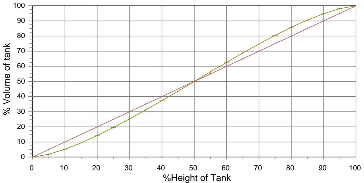
Graph 2a: Height of Liquid to Volume of Horizontal Tank
